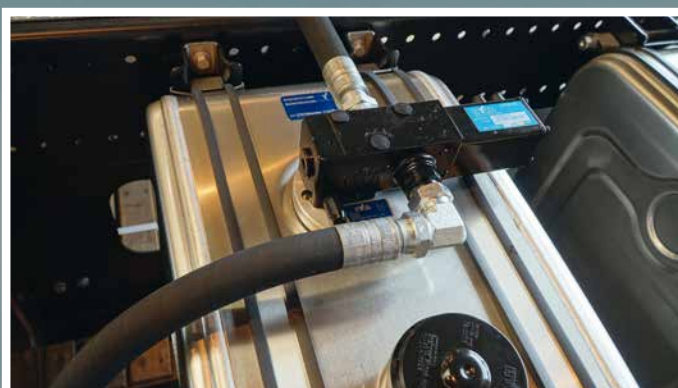
Tipping valve mounted on the return filter
